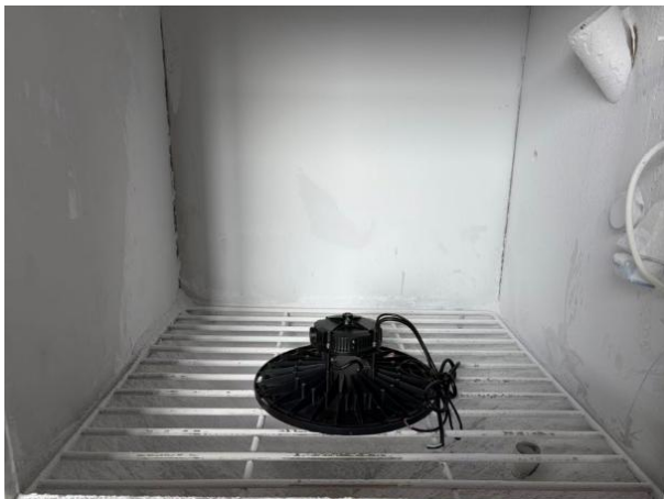
Fig.2: IP6X Pre Testing (Model: ASD-UHG-ST-240[BK,WH]-[BLANK,EM])
