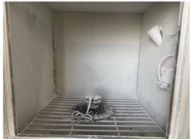
Fig.3: IP6X Post Testing (Model: ASD-UHG-ST-240[BK,WH]-[BLANK,EM])
