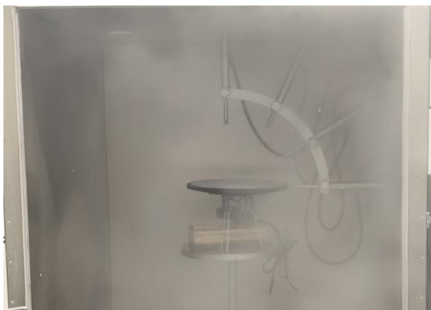
Fig.4: IPX9K Testing (Model: ASD-UHG-ST-240[BK,WH]-[BLANK,EM])
