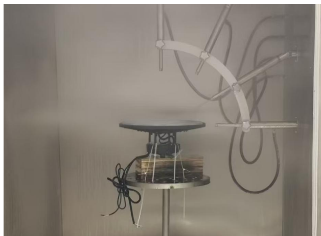
Fig.5: IPX9K Testing (Model: ASD-UHG-ST-240[BK,WH]-[BLANK,EM])
