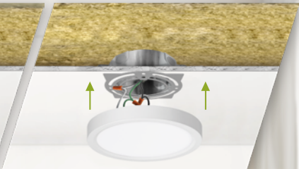
JUNCTION BOX INSTALLATION
